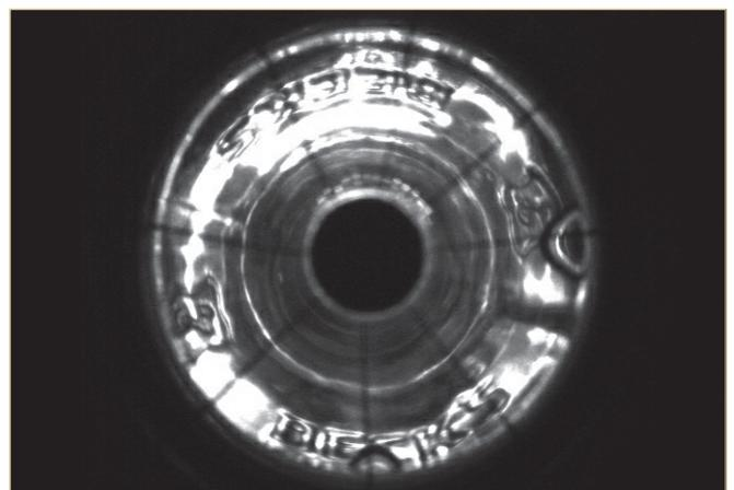
Using one hypertelecentric lens for each row of bottles, embossing can now be fully detected and analysed, even on the steep neck section, and this happens precisely when each bottle is positioned concentrically under the lens to achieve optimum image results.
