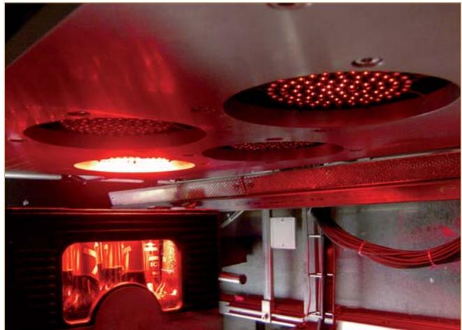
Using a patented ultra-compact, high-performance LED illumination system, embossing on bottles is visible with a strong image contrast.
